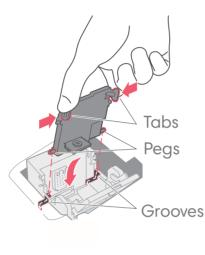
d. Squeeze the tabs and slide the Printhead pegs into the lower set of grooves.
