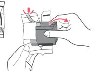
e. Keep squeezing the tabs and f. Unwrap the Ink Cartridge push the Printhead flat against the and make sure you remove the wall. The tabs will click open when silver foil strip. placed correctly.
