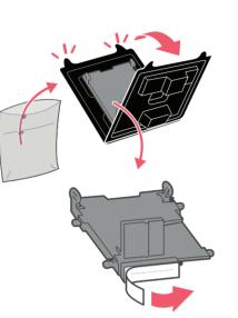
b. Remove the packing tape from the ink carriage and open the guard.
