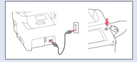
Connect your machine to a power source and turn on the power
