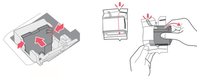
e. Keep squeezing the tabs and push the Printhead flat against the wall. The tabs will click open when placed correctly.
