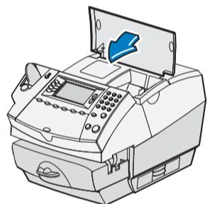
5.9 Close the top cover. The franking machine will now go through a setup cycle which takes up to 2 minutes.
