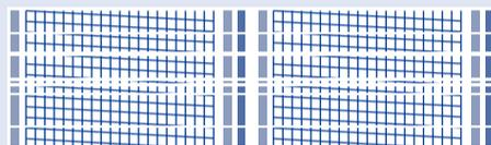
**Bad print** - broken lines in the centre of the test print
