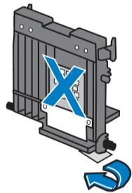
4.3 Remove the print head from its packaging and peel the tape strip from the print head. **DO NOT** touch the contacts on the print head.
