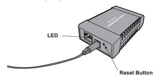
c. Wait another 45 seconds for the Communication Device to complete its startup routine. When the LED is blinking in a regular pattern (typically Orange, Green, Orange, Green, Pause), continue with step 2 below.
