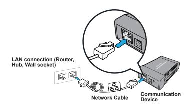
Plug the AC power adapter into the Communication Device and a power outlet. The left LED is lit yellow when it is on.
