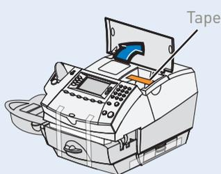
3.1 Open ink access cover and remove tape and shipping material.
