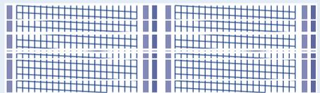
**Bad print** - broken lines in the centre of the test print
