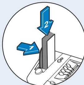
3.4 Push the tape lever to the right and drop tapes into the slot. The printable side of the tape should be facing towards the right.
