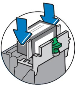
5.7 Insert the cartridge. The ridges on the cartridge slide into the grooves.
