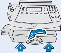
3.3 Close feed deck by lifting it and rotating clearance lever anticlockwise.
