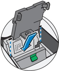
5.4 Slide the print head pegs down into the grooves.
