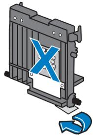
5.3 Remove the print head from its packaging and peel the tape strip from the print head. **DO NOT** touch the contacts on the print head.
