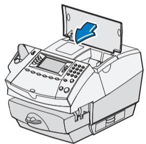
5.9 Close the top cover. The franking machine will now go through a setup cycle which takes up to **2 minutes**.
