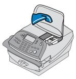
4.9 Close the top cover. The franking machine will now go through a setup cycle which takes up to 2 minutes.
