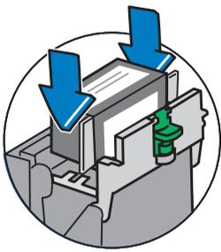
4.7 Insert the cartridge. The ridges on the cartridge slide into the grooves.
