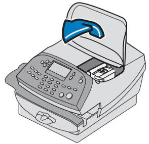
4.9 Close the top cover. The franking machine will now go through a setup cycle which takes up to **2 minutes**.
