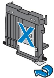
4.3 Remove the print head from its packaging and peel the tape strip from the print head. DO NOT touch the contacts on the print head.
